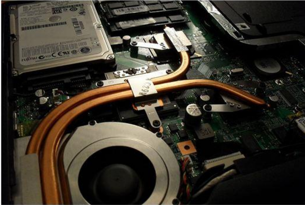
Figure 2 Heat pipes in a laptop computer
